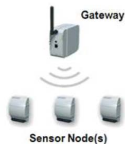
Fig. 1: WSN Components, Gateway, and Distributed Nodes
